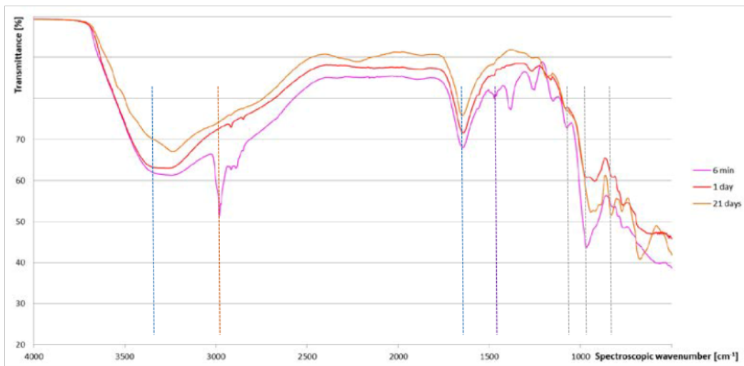
Figure 8: FTIR time dependence of AAM dried at room temperature. Blue lines O-H bonds, orange lines C-H bonds, dashed purple lines aromatic C-H 2 and C-H 3 bonds, grey lines Si-O bonds.
