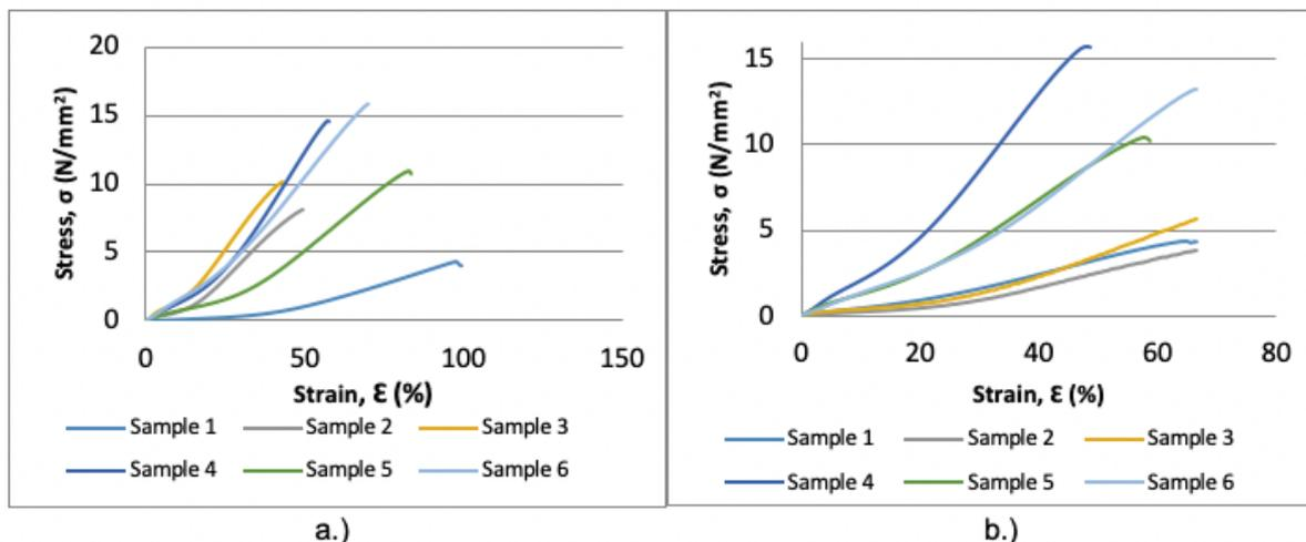
**Figure 4.** Stress/strain curves of samples in the longitudinal (a) and transverse (b) directions (wet condition)
