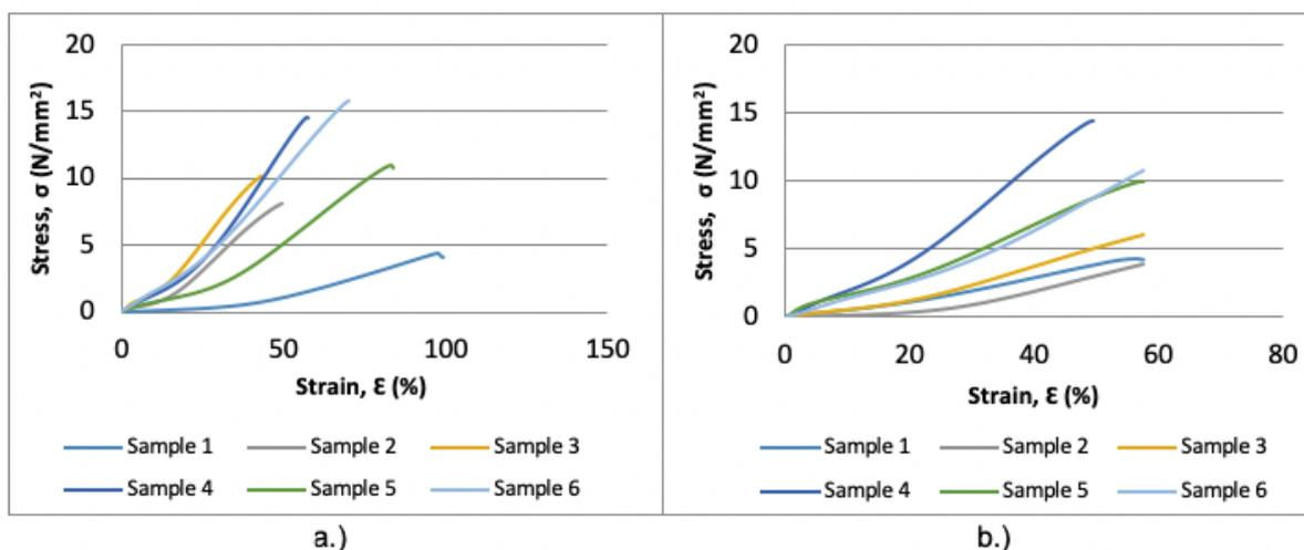
**Figure 3.** Stress/strain curves of samples in the longitudinal (a) and transverse (b) directions (dry condition)
