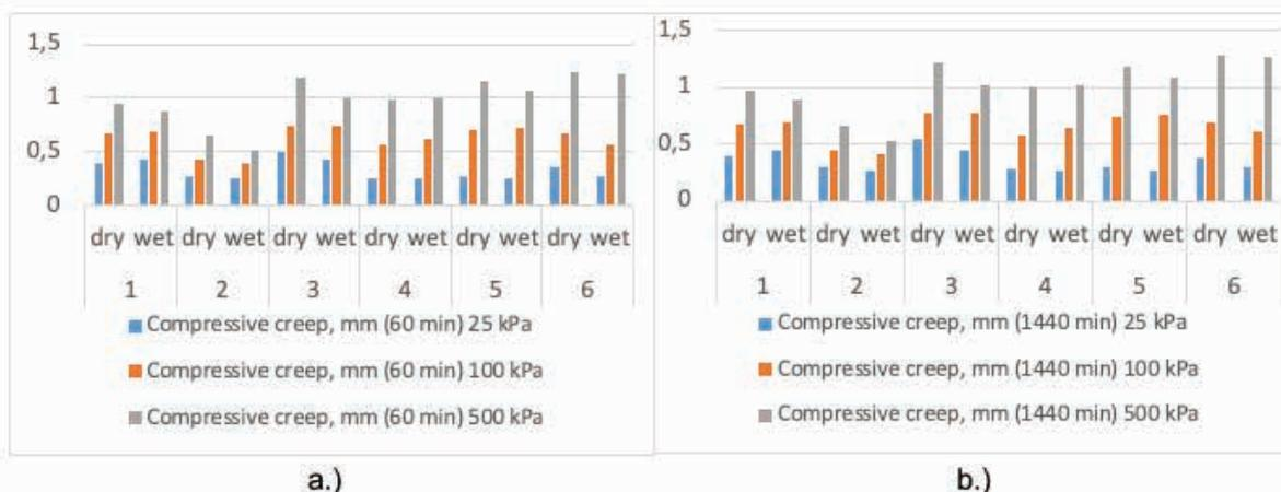
Figure 5. Compressive creep after 60 minutes (a) and 1440 minutes of compressive loading (b)
