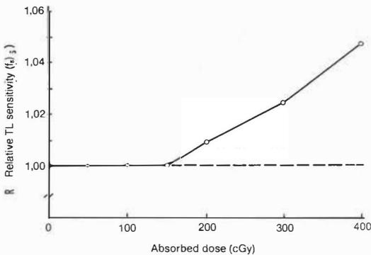
Fig. 5 — The effect of exposure on relative TL sensitivity ( $f_e$  in equation 2).
