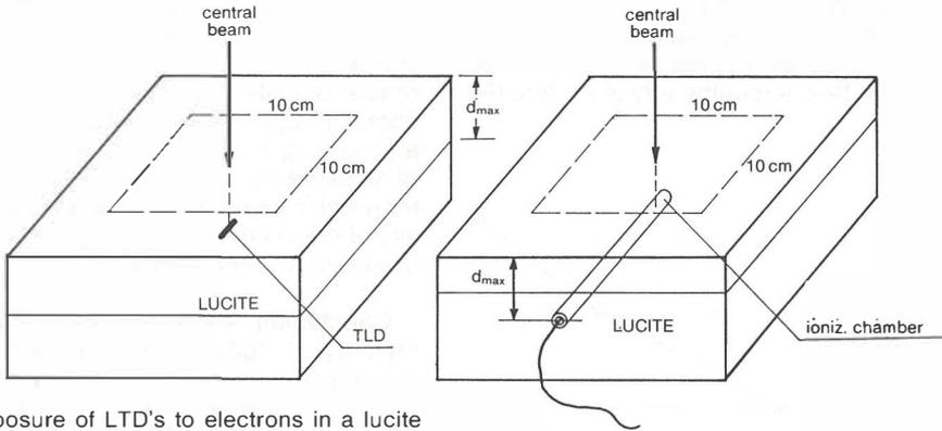
Fig. 3 — Exposure of TLD's to electrons in a lucite phantom (a). Determination of absorbed dose with Farmer ionization chamber.  $d_{max}$  is the depth of maximum absorbed dose for electrons with energy selected (b).
