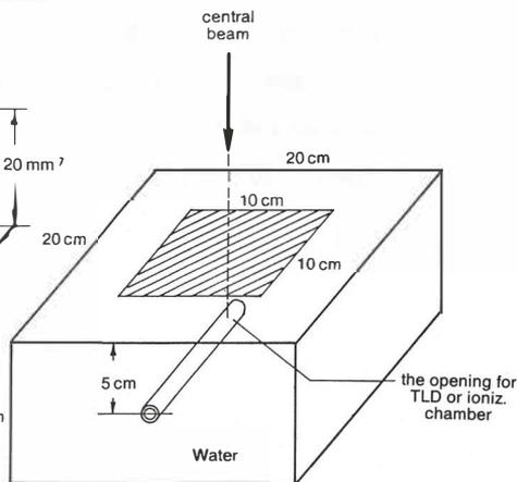
Fig. 2 — Exposure of TLD to Co<sup>60</sup> gamma rays and 8 MeV x-rays in a water phantom.
