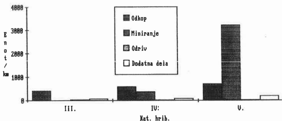
Slika 13: Struktura stroškov pri izvedbi spodnjega ustroja (Naklon terena 40%) Figure 13: Cost structure in the road-bed construction (with a 40%-terrain slope)
