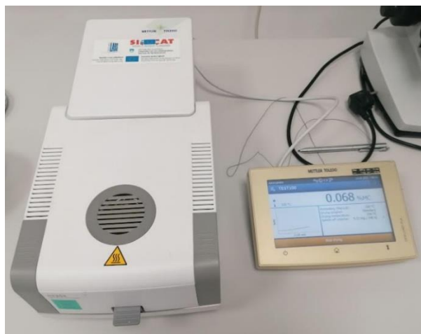
Slika 16: Analizator vlage Mettler Toledo, HX024
