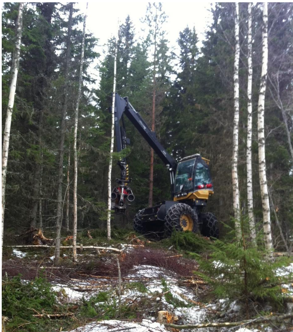
Figure 48: Commercial (first) thinning of a mixed conifer-deciduous stand using a small 4 wheeled harvester in northern Sweden in November 2017. Commercial thinning is performed yearly on over 300,000 ha in Sweden, Pulpwood is typically the main product produced during commercial thinning (© Back Tomas Ersson, SLU).
