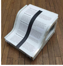
Fig. 7. The dummy object of inspection with a line standing in for an edge, and random text around for a random background.
