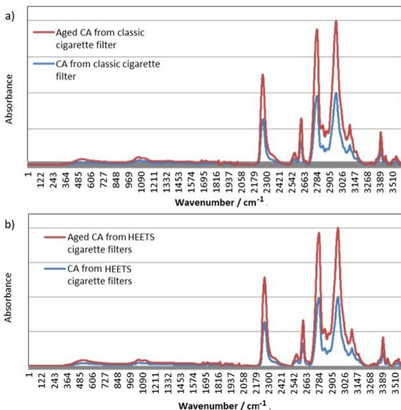
**Figure 2.** FTIR spectra of CA microplastics from used cigarette butts (a) from classic cigarette filters and (b) from HEETS filters.
