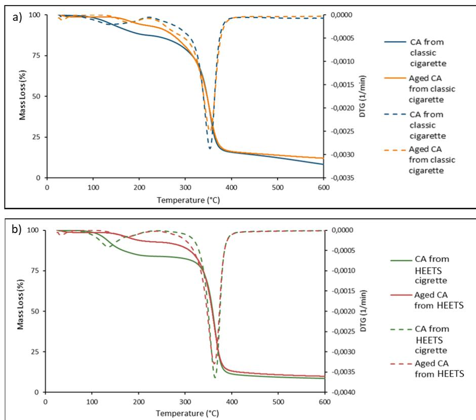
**Figure 3.** TGA/DTG analysis of unaged and artificially aged (a) CA classic and (b) CA HEETS cigarette filters.
