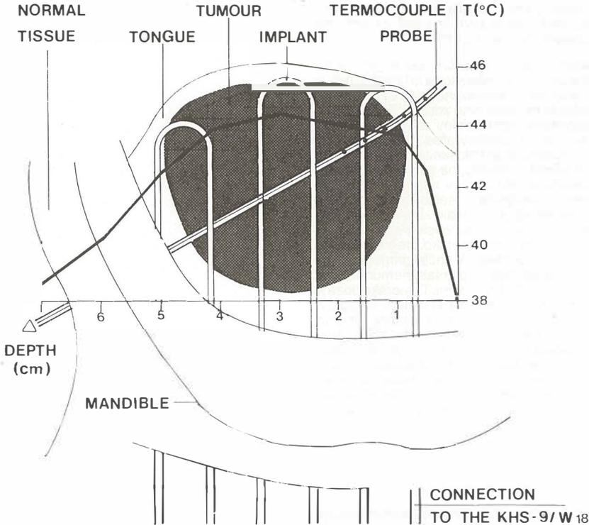
Fig. 4 — Schematic presentation of tumor implant in the mobile tongue. There is a plastic tube inserted obliquely through the tumour centre used for passing of the movable termister probe. The arrow indicates the movement direction. Superposed graph shows the temperatures measured in that region.
