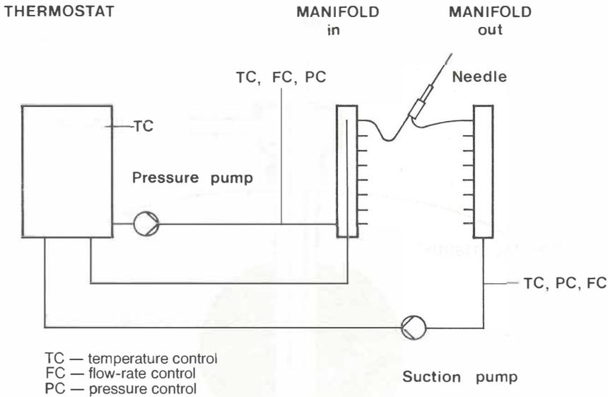
Fig. 1 — Schematic presentation of the KHS-9/W 18 hyperthermia unit
