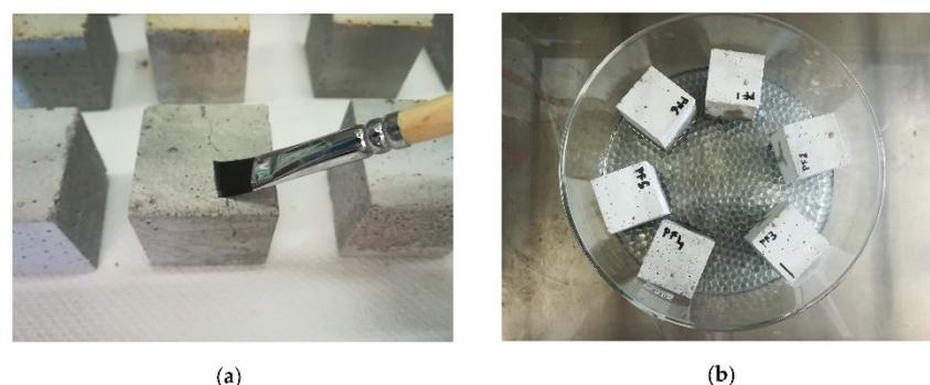
**Figure 2.** Example of application procedures of CFW: (a) brush till refuse, AP1; (b) absorption through capillarity, AP2.
