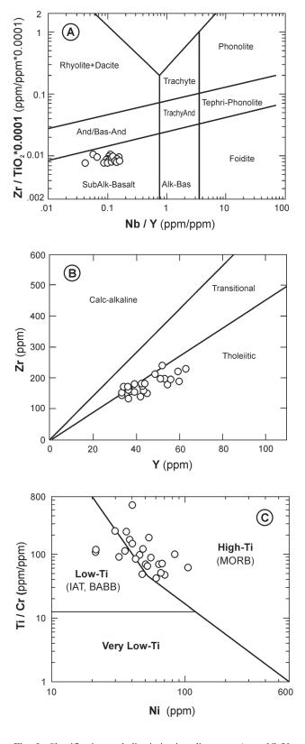
Fig. 9. Classification and discrimination diagrams:  $A - Nb/Y - Zr/TiO_2*0.0001$  (Winchester & Floyd 1977); B - Y - Zr (Barrett & MacLean 1994); C - Ni - Ti/Cr (Beccaluva et al. 1983) for the ortho-greenschists from Mt. Medvednica metamorphic complex. IAT=island-arc tholeiites, MORB=mid-ocean ridge basalts, BABB= back-arc basin basalts.
