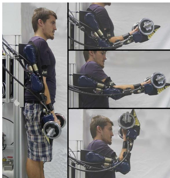
Fig. 1. Images of a human wearing an exoskeleton and holding a weight in four different arm configurations.
